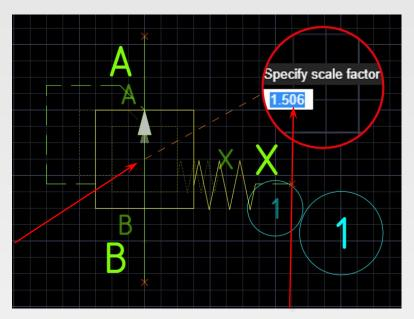
Select a base point and move cursor to resize Alternatively, define the scale factor in the text box for precise scaling
